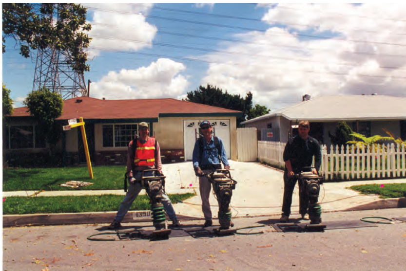
Tom Pratt (USGS), James Dolan (USC) and John Shaw (Harvard) collecting high-resolution seismic reflection data above the central, Santa Fe Springs segment of the Puente Hills thrust (see Pratt et al., 2002 (BSSA); Shaw et al. 2002 (BSSA); and Dolan et al., 2004 (Science)).
